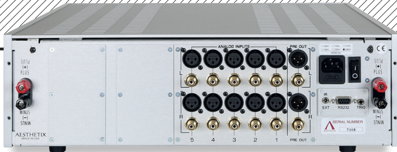
ABOVE: Pictured here in its most basic form – note blanks in place over optional MM/MC phono bay [far left] and digital input bay [left] – the Mimas offers five line inputs and one pre-out (on RCAs and XLRs) plus fully floating 4mm speaker terminals
